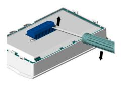
Fig. 4 If needed, remove the terminal strip by sliding it up and off the thermostat body
