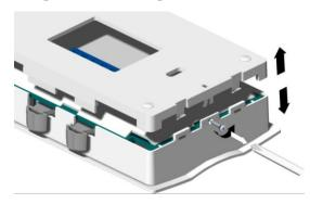
Fig. 2 Taking out back plate
