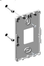
Fig. 3.Installing back plate
